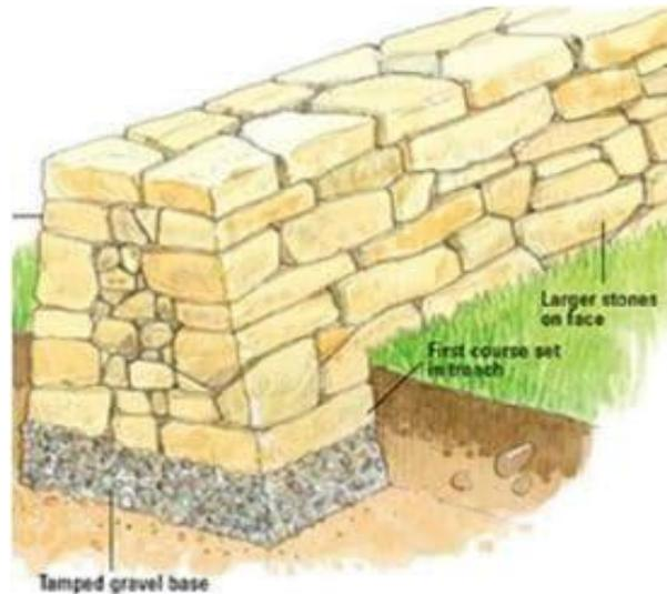
Fig.1.19: Dry Rubble Masonry
