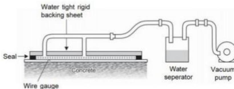
Fig 2.3 Vacuum Dewatered Flooring
