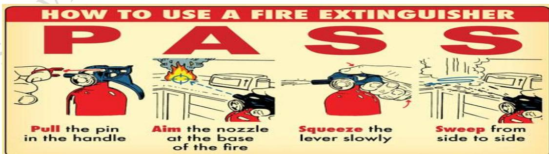
**Fig 3.3 Use of Fire Extinguisher**
