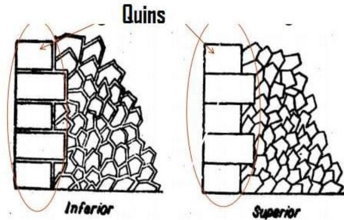
Fig.1.18: Polygonal Rubble Masonry
