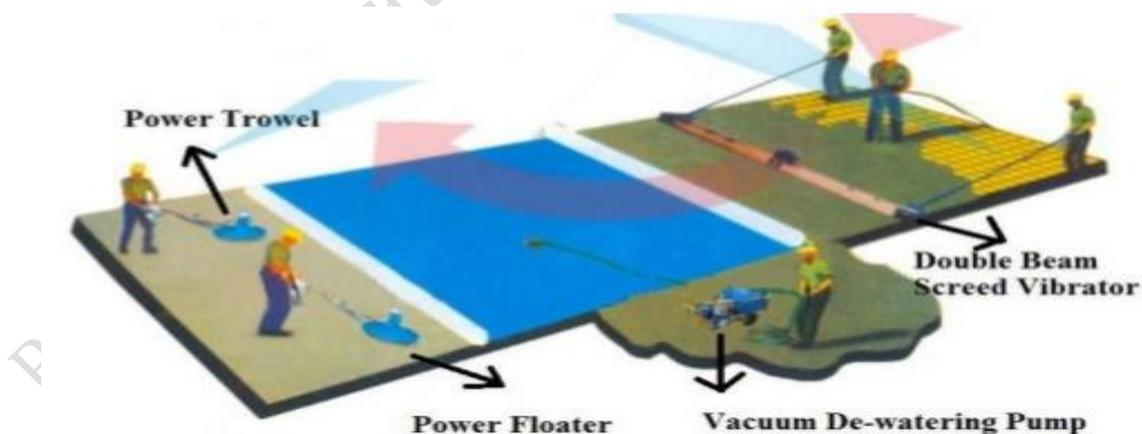
Fig 2.13 Tremix Vacuum System Stages
