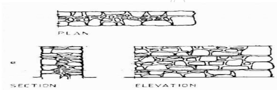
Fig.1.15: Coursed Rubble Masonry
